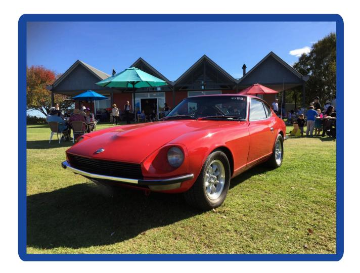
Photo of my Datsun 240Z, 1972. Engine has a high lift cam, high compression head, triple Dellorto dlha40 carbs and extractor exhaust. Suspension has been lowered 50mm. Alloy wheels are from Performance Wheels originally made here in Adelaide.
